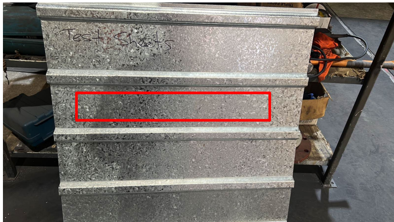
Figure 1. Test sample as received. The red box shows location of the tested section.
